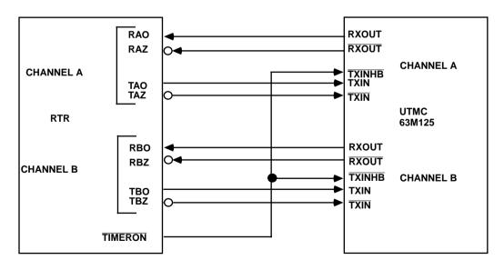
Figure 20b. RTR Transceiver Interface Diagram
