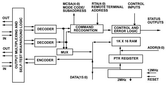
Figure 1. UT1553B RTR Functional Block Diagram
