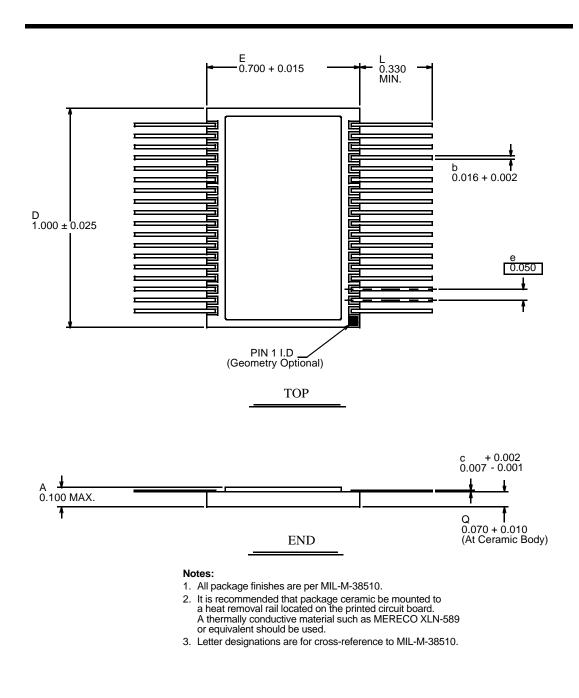
36-Lead Flatpack, Dual Cavity (50-MIL Lead Spacing)
