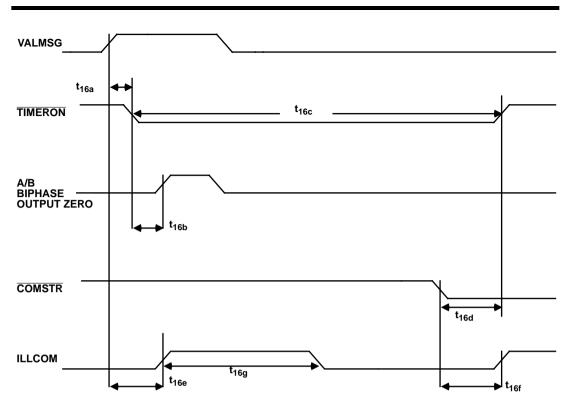
Figure 16. RT Fail-Safe Timer Signal Relationships
