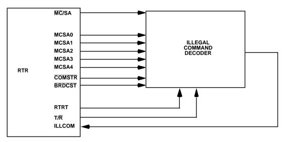
Figure 21. Mode Code/Subaddress Illegalization Circuit
